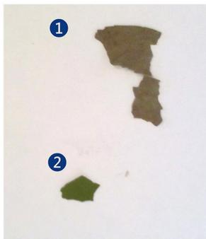
① AII Green sample from the wing root (highly worn, exposed to elements) of 13-42.
