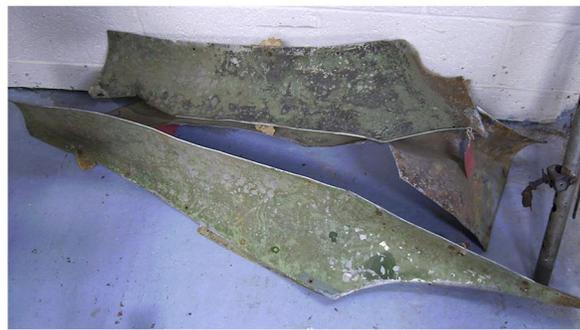
The port wing root fairing of 13-42 next to the starboard unit from a Yak-7B finished with AMT paints (alas, p/n currently unknown). The two greens are evidently different to the naked eye, even upon casual inspection.
